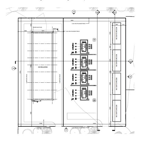
Picture 09 | Proposed ESB Substation Compound Plan The substation development is to be made of two elements, the first being a new node on the Irish electricity grid at Naas, which will be handed over and be operated by EirGrid ESO as the transmission system operator (TSO); the second element will comprise the transformation to a lower voltage to enable distribution to the new proposed data centre development.
